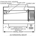
(H) HORIZONTAL MOUNT HORIZONTAL MOUNTING MODELS INCLUDES STAINLESS STEEL NEGATOR SPRINGS AND BLADE LOCKS
