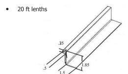
Intermediate reinforcement for rectangular duct. Fasten with 3/4" of vertical duct wall and then 8" on center.
